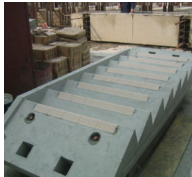
Figure 123 Precast staircases (Source: Hong Kong Housing Authority)
