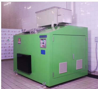
Figure 150 Food waste decomposer in Olympian City, West Kowloon (Source: Sino Group)
