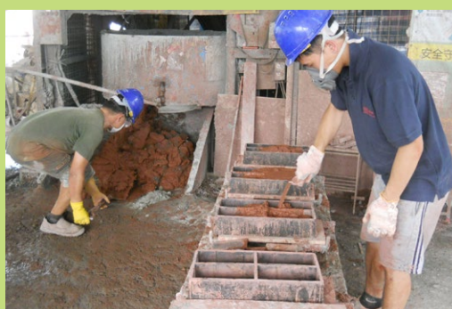
Figure 127 Recycling of marine mud (Source: Hong Kong Housing Authority)
