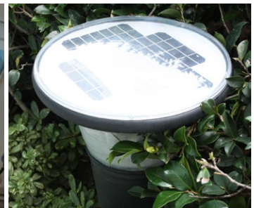
Figure 117 Solar lawn lamps, automatically switch on at night and only use solar (Source: Kai Shing Management Services Limited)
