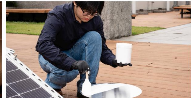
The water-soluble SARC coating can also be produced in various colours, allowing it to be easily applied to building roofs, walls, roadways, and urban surfaces to achieve both cooling and aesthetic enhancements.
